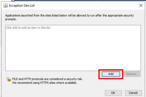
The following exception can be added as the Ether IO24 TCP can be configured to a fixed IP address by placing jumper four on the board; any other IP can be added once configured. NOTE: make sure that the IP address and the subnet mask are within the same subnet to allow for communications between the Ether IO24TCP and the computer.
