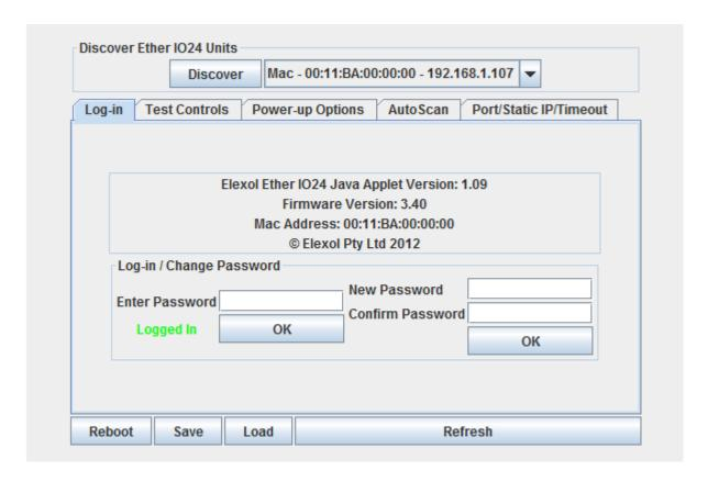
2. Log into unit and Click the Auto scan Setup tab to fill in the autoscan setup values
