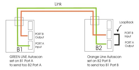
The above picture shows an example of two Ether IO24's connected together without a need for a PC interface. It also shows how the system can be used to provide feedback between the two units.
