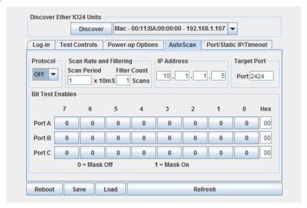
Set up the IP address and Port number for the target address that will be used. This may be a PC or another Ether IO24 unit.
